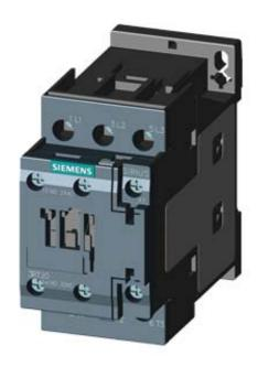
CONTACTOR, AC-3, 5.5KW/400V, 1NO+1NC, AC110V 50HZ, 120V 60HZ 3-POLE, SZ SO SCREW TERMINAL
