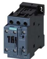
power contactor, AC-3e/AC-3, 12 A, 5.5 kW / 400 V, 3-pole, 24 V DC, auxiliary contacts: 1 NO + 1 NC, screw terminal, size: S0
