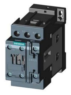
CONTACTOR, AC-3, 5.5KW/400V, 1NO+1NC, AC(50-60HZ)/DC ACTUAT. , UC 95...130V, 3-POLE, SZ S0 SCREW TERMINAL
