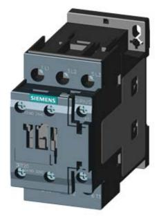
CONTACTOR, AC-3, 7.5KW/400V, 1NO+1NC, AC110V 50HZ, 120V 60HZ 3-POLE, SZ S0 SCREW TERMINAL
