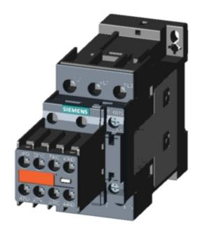
CONTACTOR, AC-3, 7.5KW/400V, 2NO+2NC, DC 24V, W. PLUGGED-IN DIODE ASSEMBLIES 3-POLE, SZ SO SCREW TERMINAL PERMANENT AUX. SWITCH
