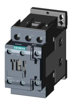
CONTACTOR, AC-3, 11KW/400V, 1NO+1NC, AC 230V 50HZ, 3-POLE, SZ SO SCREW TERMINAL
