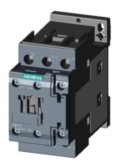
CONTACTOR, AC-3, 18.5KW/400V, 1NO+1NC, AC 230V 50HZ, 3-POLE, SZ SO SCREW TERMINAL
