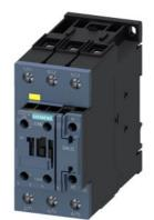
power contactor, AC-3e/AC-3, 51 A, 22 kW / 400 V, 3-pole, 21-33 V AC/DC, 50/60 Hz, with integrated varistor, auxiliary contacts: 1 NC, screw terminal, F-PLC-IN
