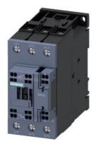
power contactor, AC-3 51 A, 22 kW / 400 V 1 NO + 1 NC, 24 V DC with varistor spring-loaded terminal suitable for 2 A PLC outputs
