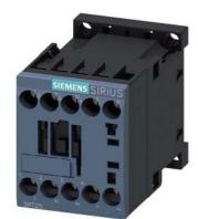
Power contactor, AC-3 9 A, 4 kW / 400 V 2 NO + 2 NC 230 V AC, 50/60 Hz 4-pole Size S00 Screw terminal
