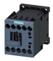
Power contactor, AC-3 9 A, 4 kW / 400 V 2 NO + 2 NC 24 V DC 4-pole Size S00 screw terminals
