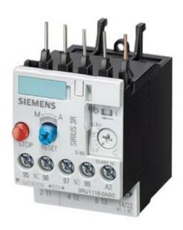
OVERLOAD RELAY, 0.7...1 A, 1NO+1NC, SIZE S00, CLASS 10, FOR CONTACTOR MOUNTING
