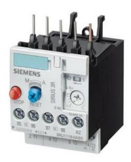
OVERLOAD RELAY, 5.5...8 A, 1NO+1NC, SIZE S00, CLASS 10, FOR CONTACTOR MOUNTING
