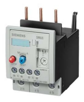
OVERLOAD RELAY, 36...45 A, 1NO+1NC, SIZE S2, CLASS 10, FOR CONTACTOR MOUNTING
