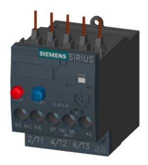
OVERLOAD RELAY 5.5...8.0 A FOR MOTOR PROTECTION SZ S00, CLASS 10, F. MOUNTING ONTO CONTACTOR MAIN CIRCUIT:
