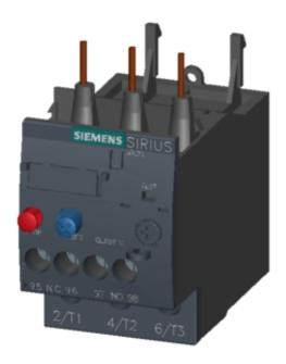
PROTECTION SZ S0, CLASS 10, F. MOUNTING ONTO CONTACTOR MAIN CIRCUIT: SCREW TERMINAL AUX. CIRCUIT: SCREW TERMINAL
