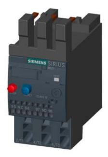
OVERLOAD RELAY 9.0...12.5 A FOR MOTOR PROTECTION BGR S0, CLASS 10 FOR MOUNTING ONTO CONTACTORS MAIN CIRCUIT: SPRING-LOADED TERMINAL AUXILARY CIRCUIT:SPRING-LOADED TERMINAL MANUAL-AUTOMATIC-RESET
