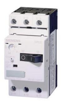
CIRCUIT-BREAKER, 0.11...0.16A N-RELEASE 2.1 A, SIZE S00 MOTOR PROTECTION, CLASS 10, SCREW CONNECTION STANDARD BREAKING CAPACITY
