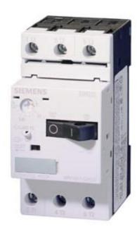
CIRCUIT-BREAKER SIZE S00, FOR MOTOR PROTECTION, CLASS 10, A-REL.0.14...0.2A,N-REL.2.6A, SCREW TERMINAL, STANDARD SWITCHING CAPACITY
