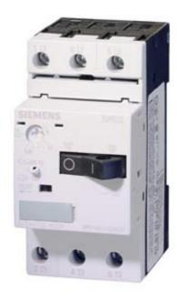
CIRCUIT-BREAKER SIZE S00, FOR MOTOR PROTECTION, CLASS 10, A-REL.0.55...0.8A, N-REL.10 A SCREW TERMINAL, STANDARD SWITCHING CAPACITY
