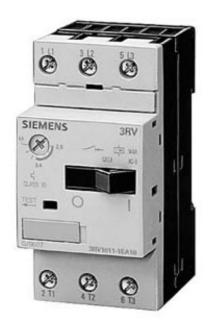
CIRCUIT-BREAKER SIZE S00, FOR MOTOR PROTECTION, CLASS 10, A-REL. 1.4...2A, N-REL. 26A, SCREW TERMINAL, STANDARD SWITCHING CAPACITY
