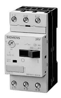
CIRCUIT-BREAKER SIZE S00, FOR MOTOR PROTECTION, CLASS 10, A-REL.1.8...2.5A, N-REL. 33A, SCREW TERMINAL, STANDARD SWITCHING CAPACITY
