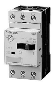
CIRCUIT-BREAKER SIZE S00, FOR MOTOR PROTECTION, CLASS 10, A-REL. 2.8...4A, N-REL. 52A, SCREW TERMINAL, STANDARD SWITCHING CAPACITY
