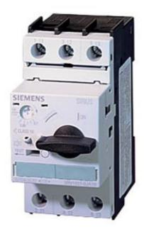
CIRCUIT-BREAKER, 0.18...0.25A N-RELEASE 3,3 A, SIZE S0, MOTOR PROTECTION, CLASS 10, SCREW CONNECTION STANDARD BREAKING CAPACITY
