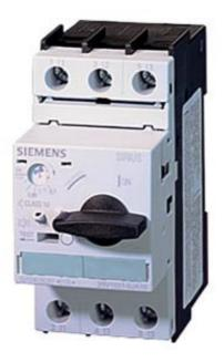
CIRCUIT-BREAKER SIZE S0, FOR MOTOR PROTECTION, CLASS 10, A-REL. 0.7 ...1A, N-REL. 13A, SCREW TERMINAL, STANDARD SWITCHING CAPACITY
