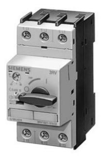
CIRCUIT-BREAKER SIZE S0, FOR MOTOR PROTECTION, CLASS 10, A-REL. 3.5...5A, N-REL. 65A, SCREW TERMINAL, STANDARD SWITCHING CAPACITY
