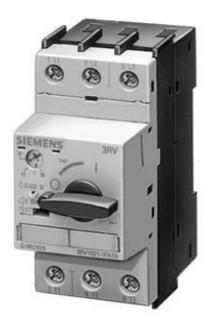
CIRCUIT-BREAKER, 14...20 A, N-RELEASE 260 A, SIZE S0, MOTOR PROTECTION, CLASS 10, SCREW CONNECTION STANDARD BREAKING CAPACITY,
