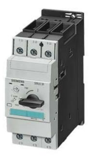
CIRCUIT-BREAKER, SIZE S2, FOR MOTOR PROTECTION, CLASS 20, A-RELEASE 11...16 A, N-RELEASE 208 A, SCREW CONNECTION, STANDARD BREAKING CAPACITY
