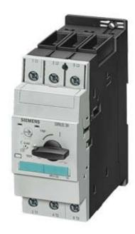
CIRCUIT-BREAKER, SIZE S2, FOR MOTOR PROTECTION, CLASS 20, A-RELEASE 22...32 A, N-RELEASE 416 A, SCREW CONNECTION, STANDARD BREAKING CAPACITY
