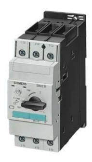
CIRCUIT-BREAKER SIZE S2. FOR MOTOR PROTECTION, CLASS 10, A-REL. 28...40A, N-REL. 520A, SCREW TERMINAL, STANDARD SWITCHING CAPACITY
