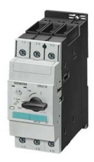
CIRCUIT-BREAKER, SIZE S2, FOR MOTOR PROTECTION, CLASS 20, A-RELEASE 28...40 A, N-RELEASE 520 A, SCREW CONNECTION, STANDARD BREAKING CAPACITY
