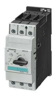
CIRCUIT-BREAKER, SIZE S2, FOR MOTOR PROTECTION, CLASS 20, A-RELEASE 36...45 A, N-RELEASE 585 A, SCREW CONNECTION, STANDARD BREAKING CAPACITY
