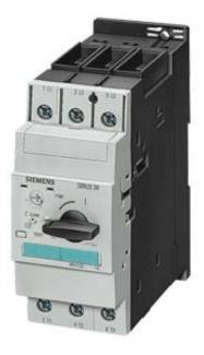
CIRCUIT-BREAKER SIZE S2. FOR MOTOR PROTECTION, CLASS 10, A-REL. 40...50A, N-REL. 650A, SCREW TERMINAL, STANDARD SWITCHING CAPACITY
