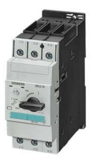
CIRCUIT-BREAKER, SIZE S2, A-RELEASE 40...50 A, N-RELEASE 650 A, MOTOR PROTECTION, CLASS 20, SCREW CONNECTION, STANDARD BREAKING CAPACITY
