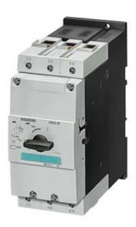
CIRCUIT-BREAKER SIZE S3 A-RELEASE 28...40 A, N-RELEASE 520 A, MOTOR PROTECTION, CLASS 10 SCREW CONNECTION STANDARD BREAKING CAPACITY
