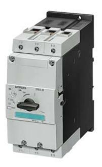
CIRCUIT-BREAKER SIZE S3, FOR MOTOR PROTECTION, CLASS 10, A-REL. 36...50A, N-REL. 650A, SCREW TERMINAL, STANDARD SWITCHING CAPACITY
