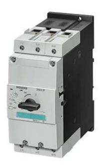
CIRCUIT-BREAKER SIZE S3 A-RELEASE 70...90 A, N-RELEASE 1170 A MOTOR PROTECTION, CLASS 10 SCREW CONNECTION STANDARD BREAKING CAPACITY
