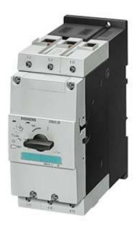
CIRCUIT-BREAKER SIZE S3 A-RELEASE 70...90 A, N-RELEASE 1170A, MOTOR PROTECTION UP TO 100 KA, CLASS 20, SCREW CONNECTION INCREASED BREAKING CAPACITY
