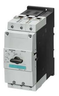
CIRCUIT-BREAKER SIZE S3 A-RELEASE 80...100 A, N-RELEASE 1235 A, MOTOR PROTECTION UP TO 100 KA, CLASS 20, SCREW CONNECTION INCREASED BREAKING CAPACITY
