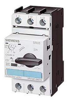
CIRCUIT-BREAKER, 2.2...3.2 A N-RELEASE 65 A, SIZE S0, TRANSFORMER PROTECTION, CL. 10, SCREW CONNECTION STANDARD BREAKING CAPACITY
