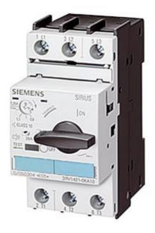
CIRCUIT-BREAKER, 4.5...6.3 A N-RELEASE 130 A, SIZE S0, TRANSFORMER PROTECTION, CL. 10, SCREW CONNECTION STANDARD BREAKING CAPACITY
