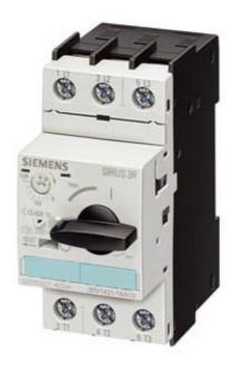
CIRCUIT-BREAKER, 9...12.5 A N-RELEASE 260 A, SIZE S0, TRANSFORMER PROTECTION, CL. 10, SCREW CONNECTION STANDARD BREAKING CAPACITY
