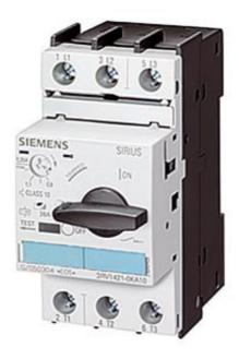
CIRCUIT-BREAKER, 11...16 A N-RELEASE 286 A, SIZE S0 TRANSFORMER PROTECTION, CL. 10, SCREW CONNECTION STANDARD BREAKING CAPACITY
