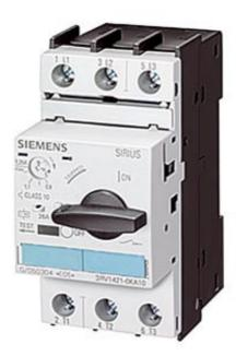
CIRCUIT-BREAKER, 14...20 A N-RELEASE 325 A, SIZE SO TRANSFORMER PROTECTION, CL. 10, SCREW CONNECTION STANDARD BREAKING CAPACITY
