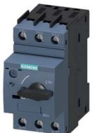
Circuit breaker size S00 for motor protection, CLASS 10 A-release 1.4...2 A N-release 26 A screw terminal Standard switching capacity
