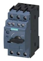
Circuit breaker size S00 for motor protection, CLASS 10 A-release 4.5...6.3 A N-release 82 A screw terminal Standard switching capacity with transverse auxiliary switches 1 NO+1 NC
