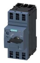
Circuit breaker size S00 for motor protection, CLASS 10 A-release 4.5...6.3 A N-release 82 A Spring-type terminal Standard switching capacity
