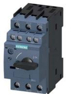
Circuit breaker size S00 for motor protection, CLASS 10 A-release 10...16 A N-release 208 A screw terminal Standard switching capacity with transverse auxiliary switches 1 NO+1 NC
