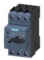
Circuit breaker size S0 for motor protection, CLASS 10 A-release 5.5...8 A N-release 104 A screw terminal Standard switching capacity
