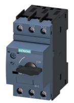
Circuit breaker size S0 for motor protection, CLASS 10 A-release 10...16 A N-release 208 A screw terminal Standard switching capacity
